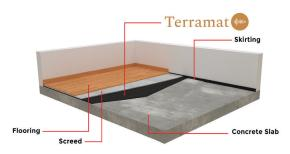
Engineered for direct adhered floor coverings such as tile, stone, wood, and vinyl floor coverings.
